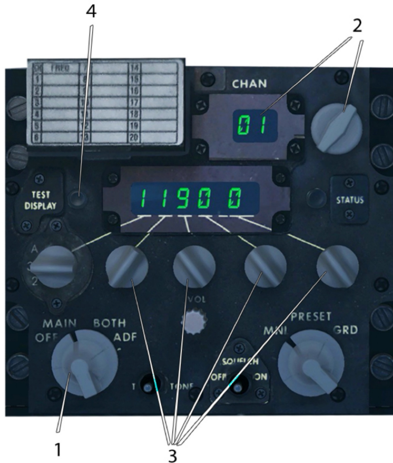
Figure 12 — Backup VHF control panel
