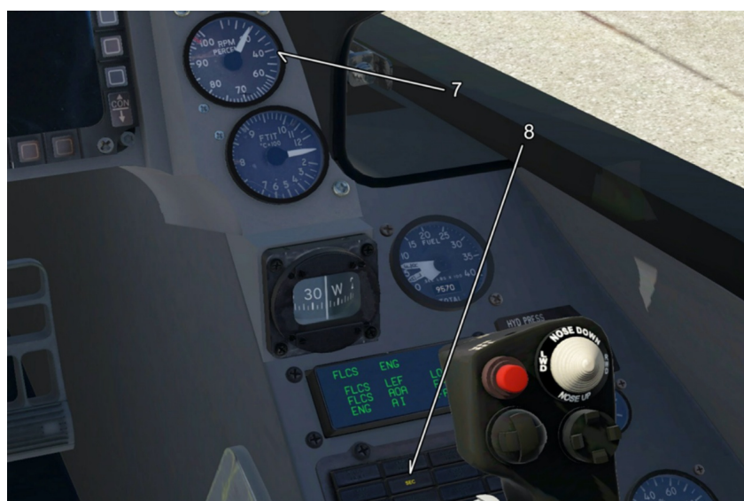
Figure 80 — Brakes, canopy and initial switches
