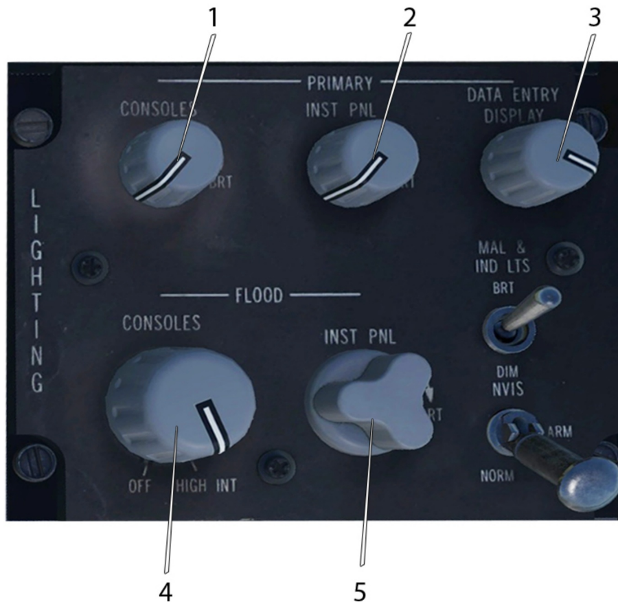
Figure 58 — Interior lighting panel
